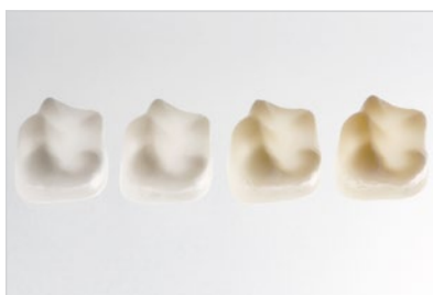
Fig 4 The translucent properties of high-strength zirconia copings are obvious when placed on a light source.
